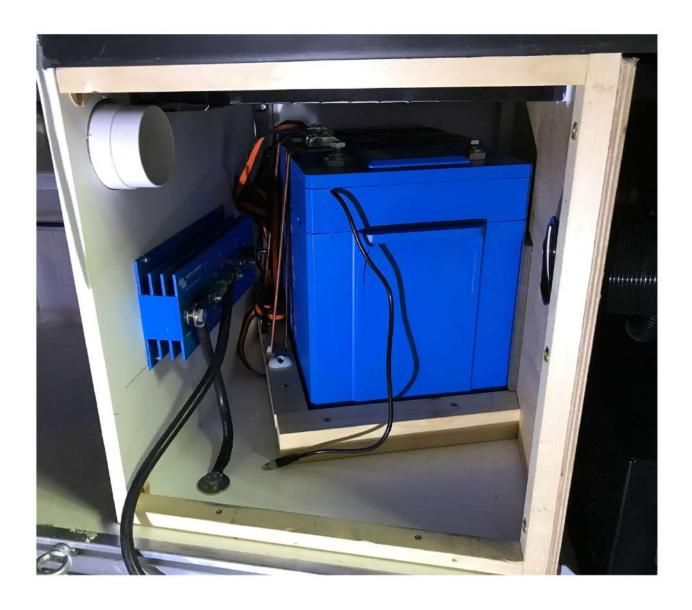
We then installed a 2 KVA Victron Multiplus and a colour control to show all the levels, charge currents and discharge currents. A Victron Battery management system was installed to regulate all the charge and discharge currents and ensure battery protection. All the cabling was calculated to ensure all the devices had the required power and the engine alternator was charging the Lithium battery whenever the vehicle engine was running.
